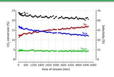
The catalytic behaviour of the 3D catalysts in the direct CO<sub>2</sub>-to-DME hydrogenation reaction (GHSV: 1,000  $NL/g_{cal}/h$ ; CO<sub>2</sub>/H<sub>2</sub>/N<sub>2</sub>: 3/9/1 v/v) was investigated at 30 bar and 200-260°C, in a tubular fixed bed reactor (i.d., 14 mm; I., 250 mm)
