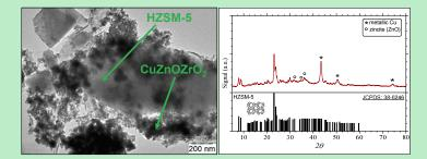
The printing procedure favours a quite uniform distribution of mixed oxides on the zeolite framework, ensuring an intimate surface contact among the phases and predicting minor restrictions in terms of transport phenomena during reaction. The intensities of the diffraction peaks at low angles (<20°) and ascribed to HZSM-5 are diagnostic of a zeolite structure well-preserved after printing and chemical interaction with metal precursors.
