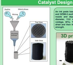
An ink paste based on Cu, Zn and Zr precursor and HZSM-5 zeolite was extruded through a thin nozzle and deposited layer-by-layer (external diameter, 13.0 mm; length, 50 mm; porosity voidage, 30%). The 3D printed structures were dried and then thermally treated for mechanical strength strength.
